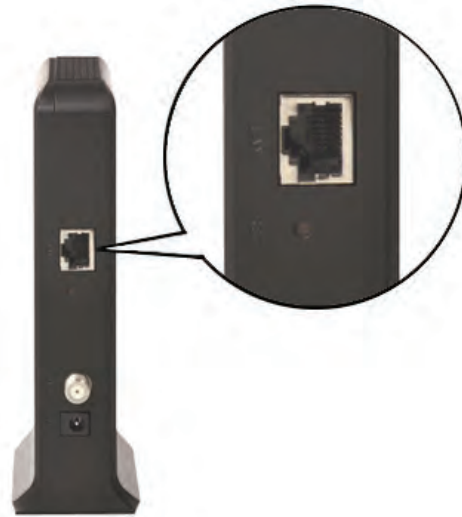
Figure 2-1. Connecting to the Ethernet Port on the Cable Modem Rear Panel
